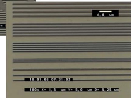
UV Nano Imprint of SUSS test structure
